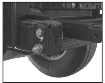
**10.** Use longer bolts (12mm-1.75 x 100mm Gr. 8.8) if no drilling is needed, slide baseplate between frame horns(If there is a gap between frame horns and baseplate insert shim as shown on front page), top bolt on each side will go inward and bottom bolt will go outward.
